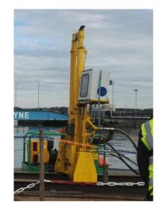
These units are supplied with a dedicated hydraulic power pack, generator and logging system. They can also be plumbed into the vessel's hydraulic system and utilise its electric supply. Beam mounted systems can be integrated into drilling masts in order to per-form CPTs within boreholes to provide a contiguous exploratory soils profile.
