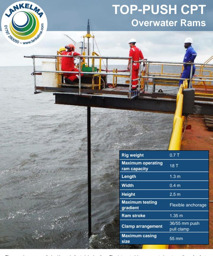
These units are supplied with a dedicated hydraulic power pack, generator and logging system. They can also be plumbed into the vessel's hydraulic system and utilise its electric supply. Beam mounted systems can be integrated into drilling masts in order to per-form CPTs within boreholes to provide a contiguous exploratory soils profile.
