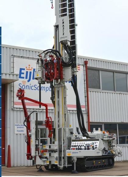
The CompactRotoSonic XL-Duo rig has a dual drill head, enabling it to carry out both sonic drilling or conventional rotary drilling (conventional or wireline) for geotechnical investigations.
