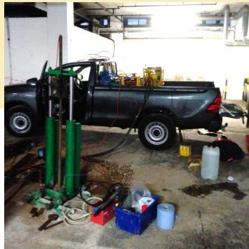
Typically, maximum penetration depth would be between 18-20m, with a push force of 18 tonne, but using the lubricating module we have reached depths of 30m with just 5 tonne of push force.
