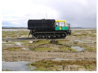
Our 'bogskipper' tracked rig's low bearing pressures, large footprint, and high ground clearance make it ideal for working sites with boggy or soft ground conditions.
