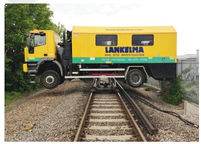
The world's first dedicated CPT rail truck, this rig can undertake multiple tests within the track's four-foot in a single possession.
