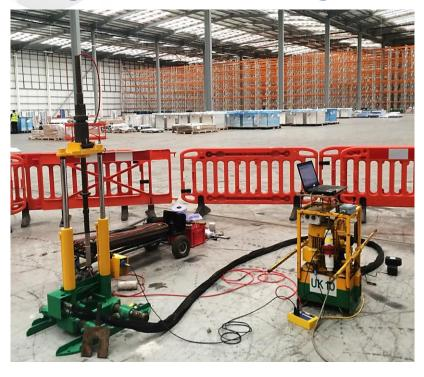
Both hand-portable rams are supported by a power pack, generator and data-logging unit, all transported in a single van mobilisation.
