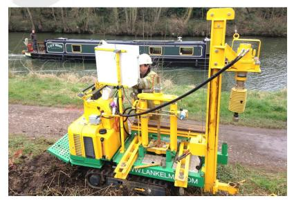
Ideal for sites with challenging access, this rig has previously been utilised in London's residences. The rubber tracks provide the rig with a low bearing pressure making it suitable for soft terrain whilst causing minimal tracking damage.
