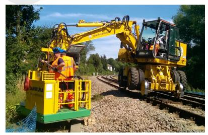
Suitable for rail investigations on embankments, cuttings, in the cess, the 4-foot and the 6-foot, and even overwater works on the edge of jack-up platforms. The reaction force is dependent on the excavator's capacity, and the CPT unit must be in contact with the ground or a solid platform to enable the push.
