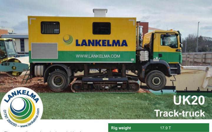
The versatile track-truck is suitable for most geotechnical sites. The rig is driven to site as a self-contained HGV with tracks that can be deployed to cope with soft or uneven terrain.
