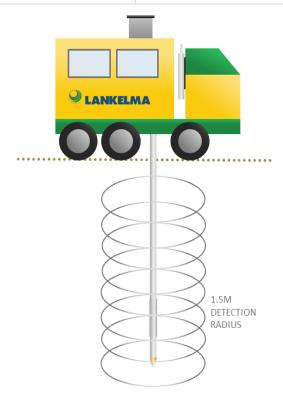
The magnetometer probe works to detect any ferrous objects in the ground by observing real-time the amplitude of the earth's magnetic field to a detection radius of 1.5m. Detection of any potential anomalies is shown as a deviation in the readings at a specified depth which can be triangulated to identify the location and depth of the anomaly.
