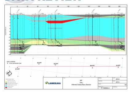
Lankelma were instructed by BP to undertake data management and quality review of data acquired by a third party CPT company in the Republic of Iraq. CPT data for 38 nr. Soundings and 74 nr. dissipation tests were sent to Lankelma for in-house processing and quality control between January and May 2014. Plots were generated to display the raw and interpreted CPT data, dissipation tests, CPT-derived liquefaction potential and fence diagrams interpolating across the site.
